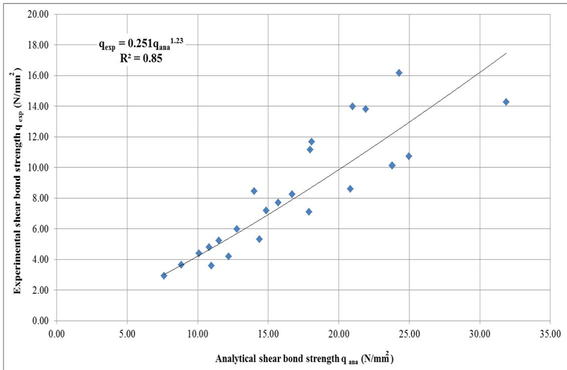
Figure 10: Relation between experimental and analytical shear bond strength
