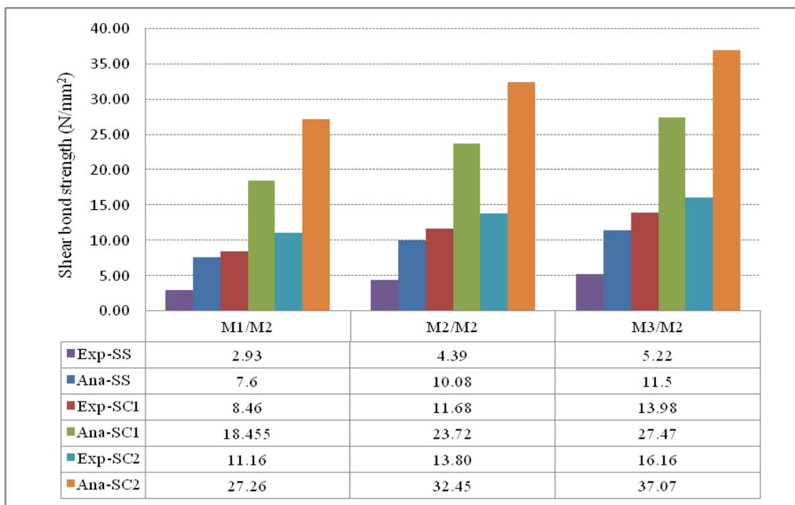
**Figure 8:** Experimental and analytical shear bond strength (N/mm<sup>2</sup>)
