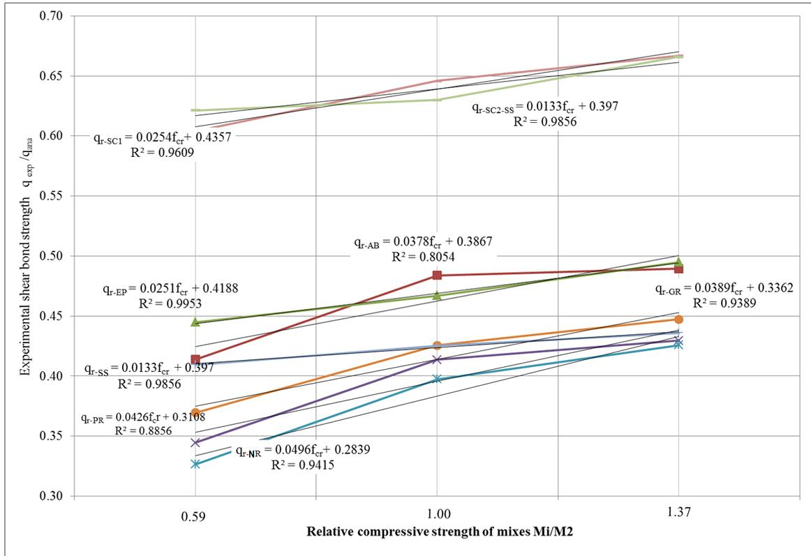
**Figure 11:** Relation between relative shear bond and compressive strength of mixes Mi/M2
