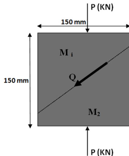
**Photo 3:** Complete specimen for slant shear test
