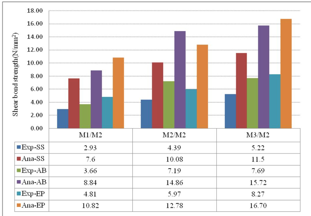
Figure 6: Experimental and analytical shear bond strength (N/mm<sup>2</sup>)
