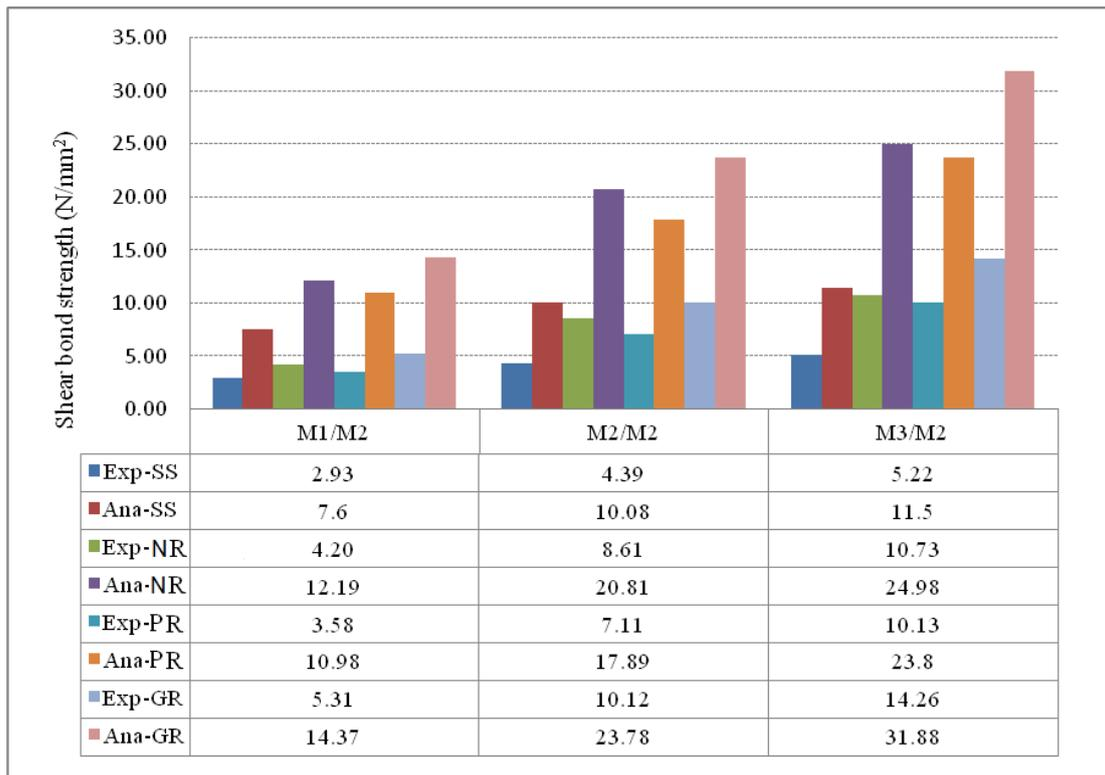
**Figure 7:** Experimental and analytical shear bond strength (N/mm<sup>2</sup>)
